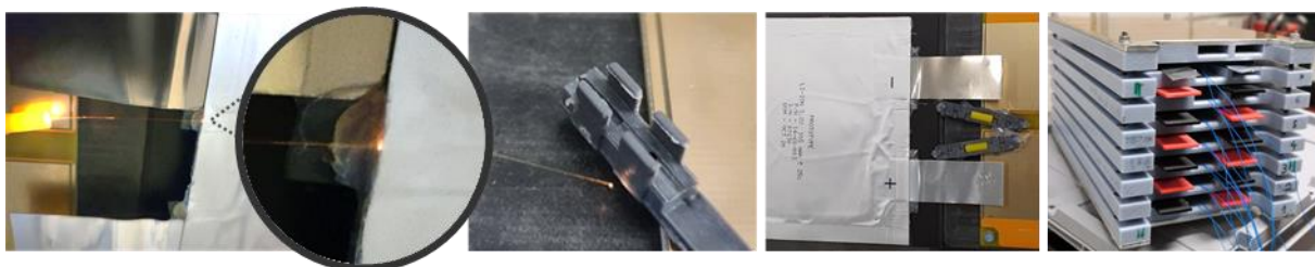
Figure 36 Fiber optic connection and connection in test stack
