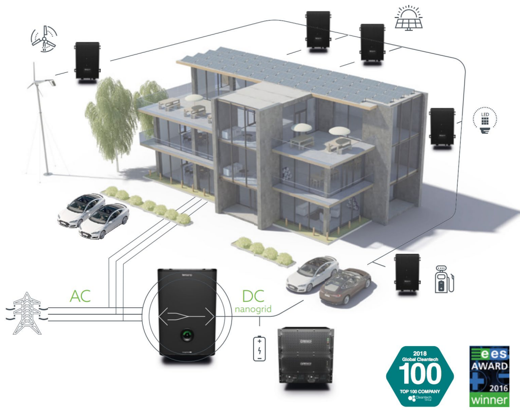
Picture: Schematic picture of Ferroamp concept with DC nanogrid; enabling to minimise DC/AC/DC losses (and costs) by using DC as much as possible and enabling DC grid between buildings. At HSB test site, this potential is not used fully as EV car charging is done with AC.
