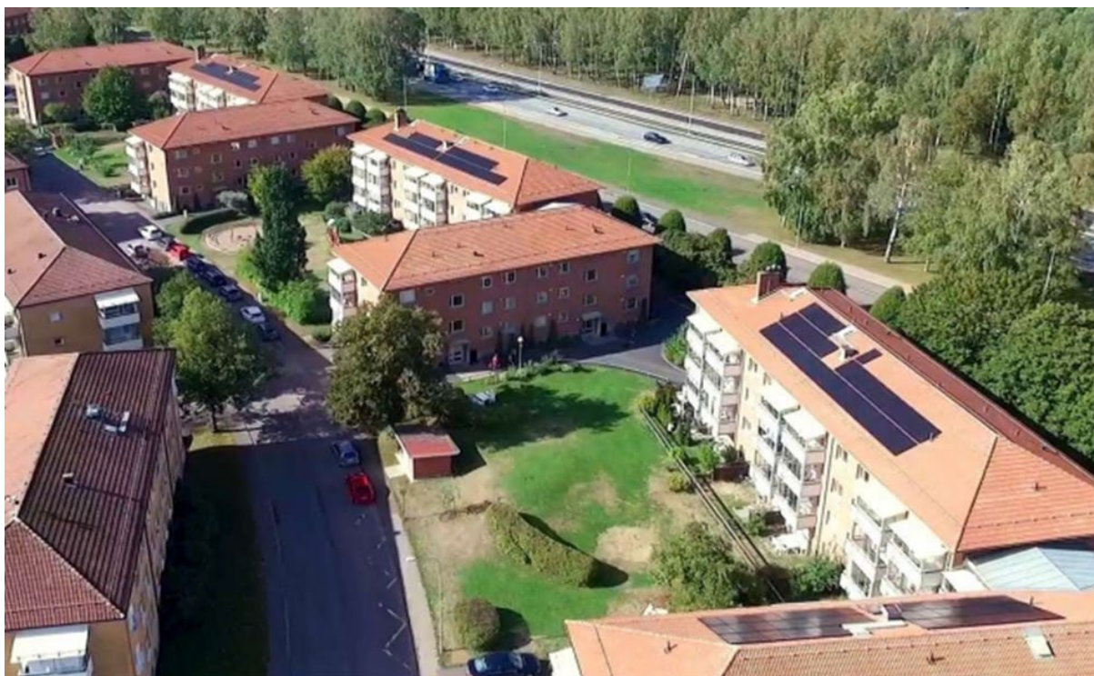
Picture: Photo of HSB Kontrollanten Housing Association with PV in two orientations
